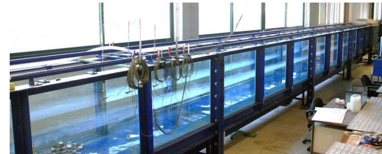
Wave Flume at DECivil, Instituto Superior Técnico, Lisbon, Portugal
